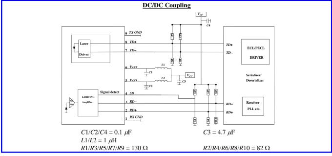
In order to get proper functionality, a recommended circuit is provided in above recommended circuit schematic. When designing the circuit interface, there are a few fundamental guidelines to follow.
