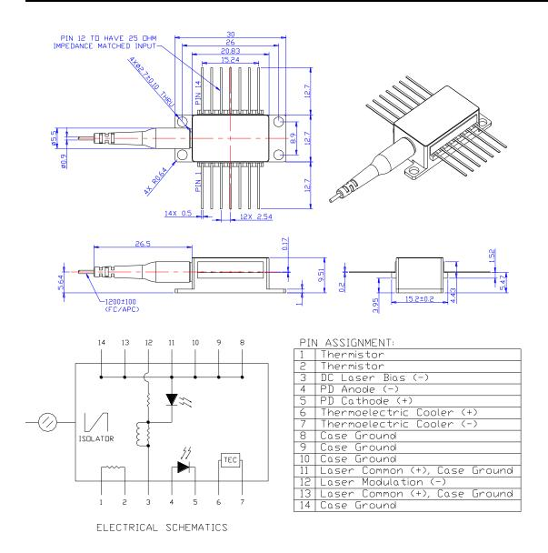
For ordering option —H2 (Negative Bias Design, Case GRD connected to LD Anode)
